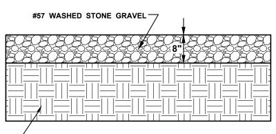
✓ TOP 12" OF SUBGRADE SHALL BE COMPACTED TO
